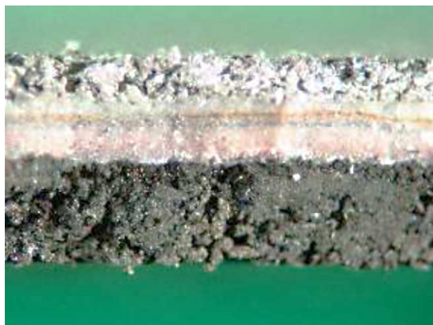
Fig. 9. Illustration of different layers that may appear in the separator layer after heating and eventual discharge. Bottom: \text{FeS}_2 positive electrode. Top: \text{Li}(\text{Al}) negative electrode.
